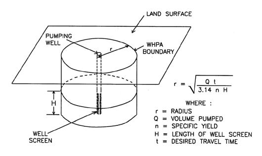
Figure 7. Calculated Fixed Radius Method
