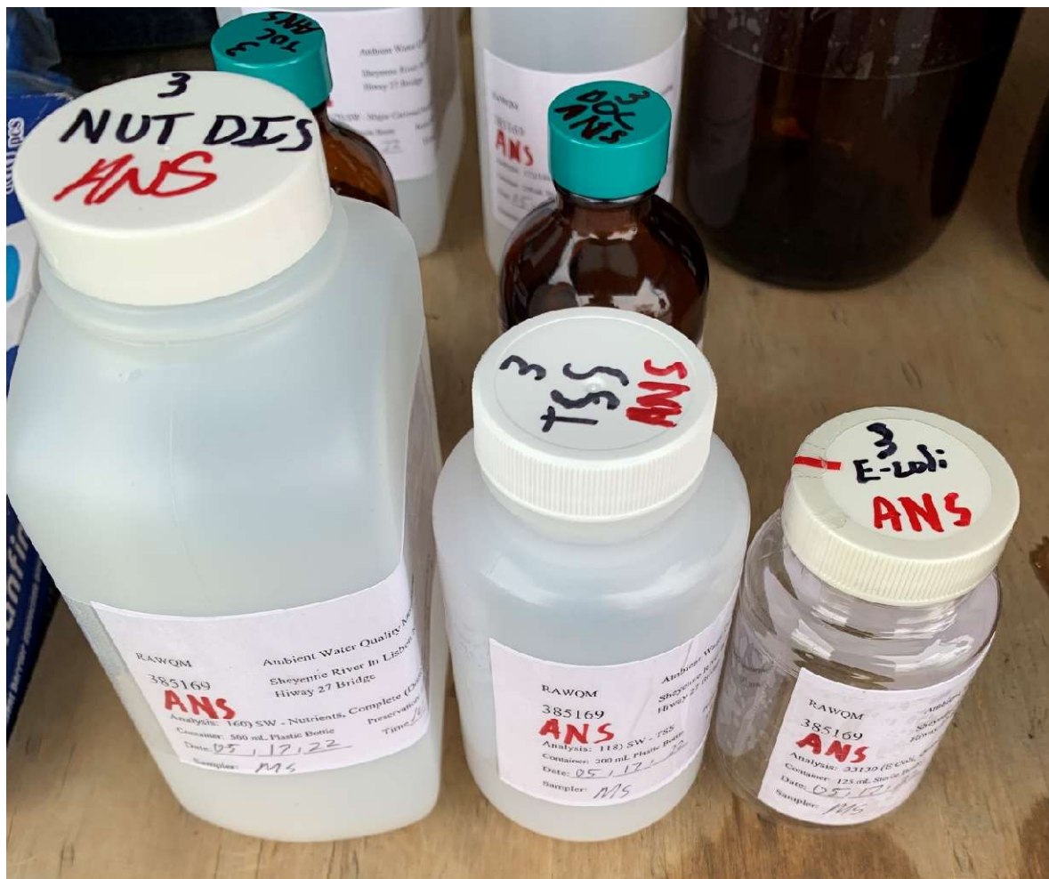
Figure 2: Properly labeled 500 ml, 250 ml and 125 ml bottles (left to right, respectively) from samples taken in a region where ANS are known to be present.
