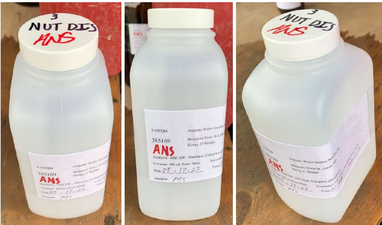
Figure 3: Properly labeled 500 ml bottle for sample taken from a region where ANS are known to be present.
