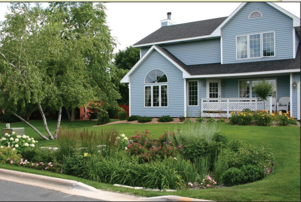
Rain gardens are shallow depressions that capture and treat stormwater naturally. Photo credit U.S. Environmental Protection Agency
