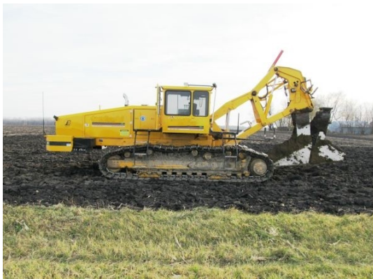
Modern tiling ploughs can be self contained or an attachment—Courtesy Alfa img.
