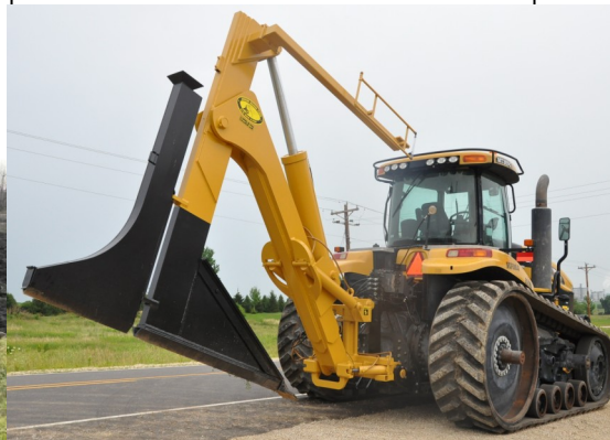
Modern tiling ploughs can be self contained or an attachment—Courtesy Alfa img.
