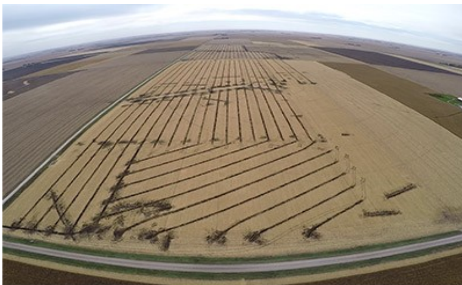
A pattern tile drainage system in a midwestern field.
