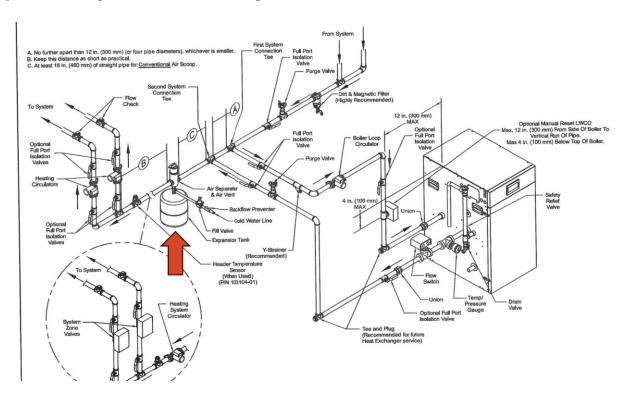
Expansion tank and air eliminator on secondary piping and suction side of circulating pumps
