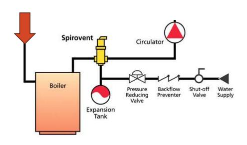
Expansion tank with air eliminator on hot side of boiler
