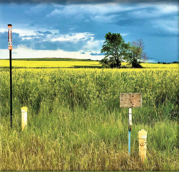
Groundwater monitoring wells (yellow pipes) are located across the state.
