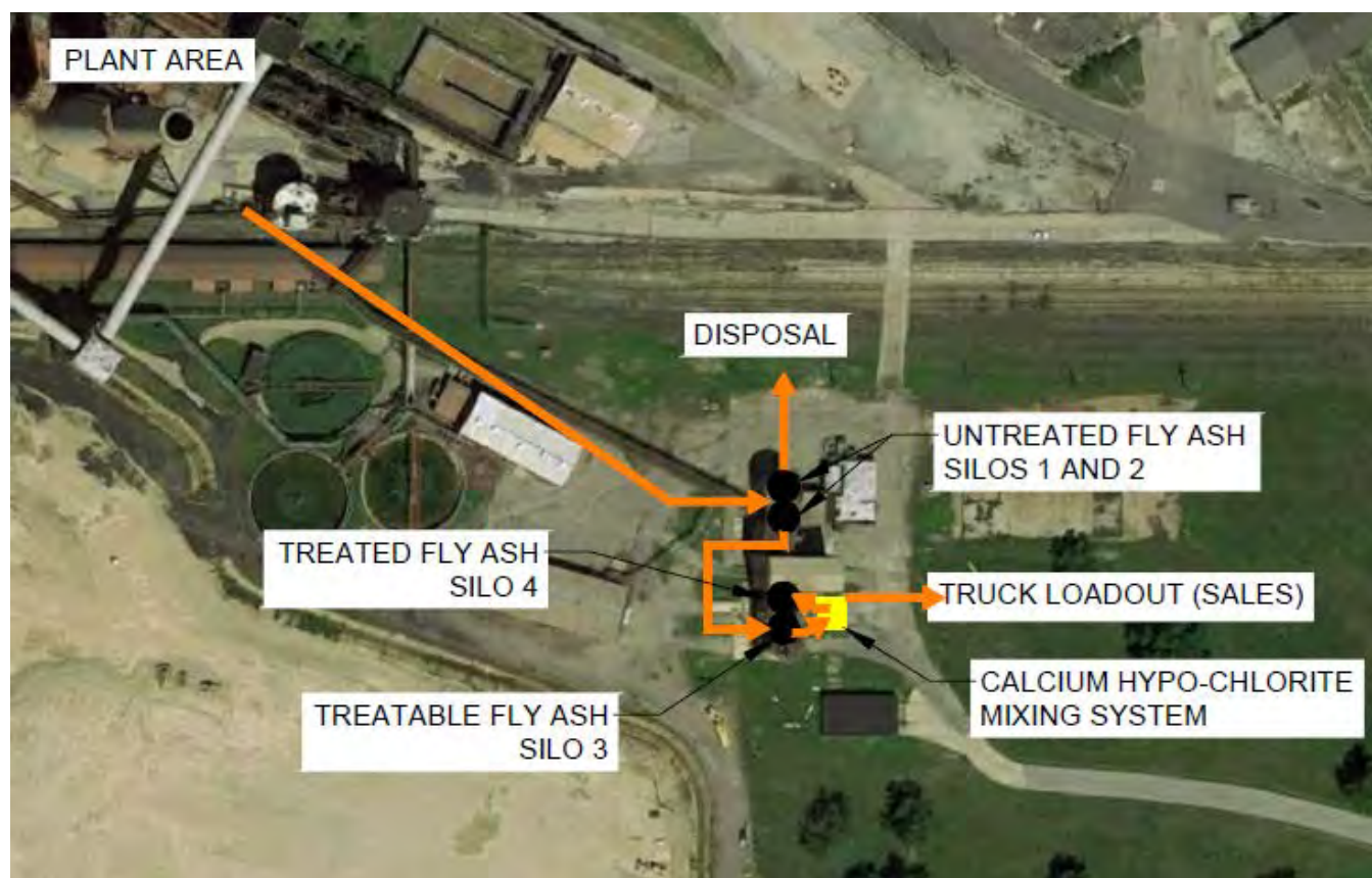
Figure 2: Eastlake Station ASM Layout
