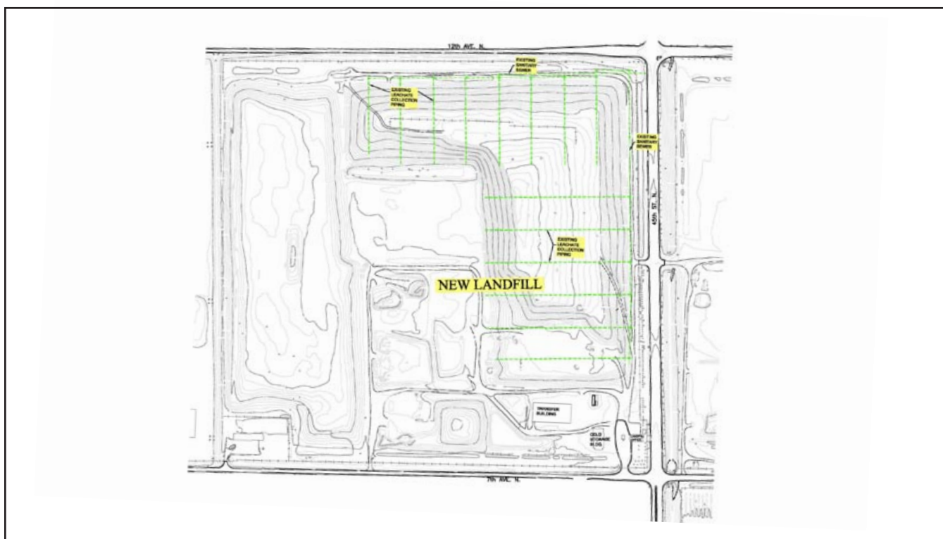
Figure 2. Landfill leachate collection system
