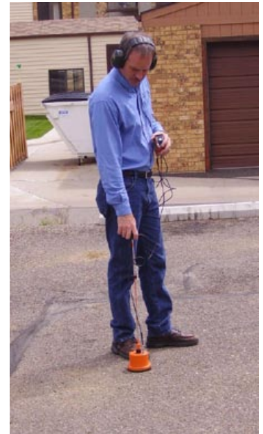
A specialized listening device can be used to help locate a water leak.
