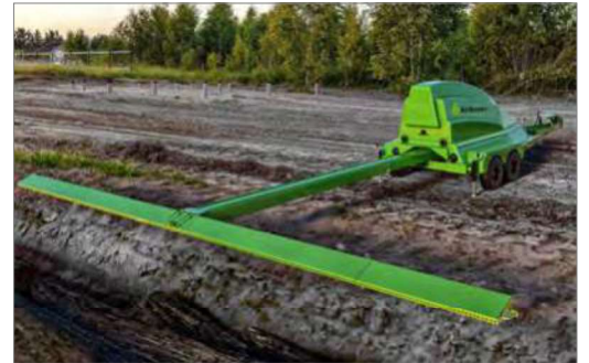
T-300 Trench Burner at Burn Pit
